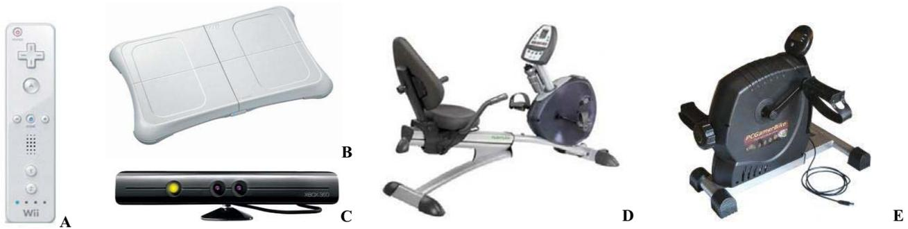
**Figure 1: Example active input hardware. (A) Wii Remote, (B) Wii Balance Board, (C) Microsoft Project Natal camera, (D) Tunturi E6R ergometer, (E) PCGamerBike Mini**
